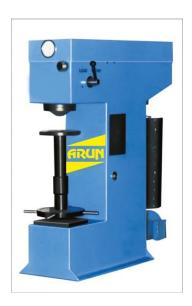
Machine designed with a hydraulic power pack and control circuit for effortless loading unloading operation. A dial gauge in front measure depth of ball penetration. This facilities production testing within tolerance limits by compression method.
